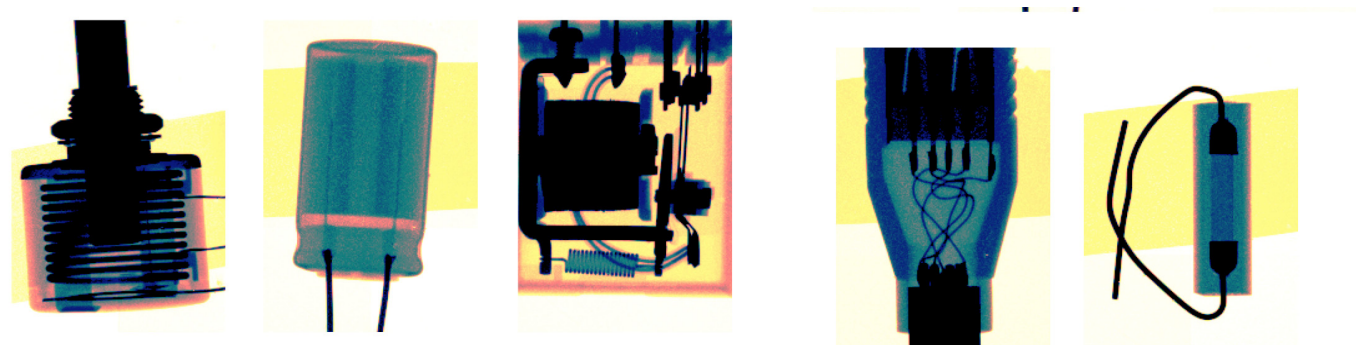
Images recorded with CdTe Hexa module with 165 \mu\text{m} pixel size.
